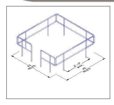
**ASP2BHR** – **Two Bar Handrail** – Is designed to be easily attached to any ASP equipment or work platform. Handrails are attached directly to the platforms by utilizing a receiver that can be welded directly to the platform or can be bolted through the grating floor using angle brackets. Handrails can be manufactured to fit any size platform.
